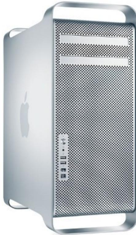
Contained in another cheap Ebay job-lot was a 2006 Apple Mac Pro. The Mac Pro was Apple's top of the line and fastest range of PC's aimed at professionals. In 2006 their possible specs were rather impressive with dual Intel Xeon multi-core processors, up to 32GB ECC memory and facility for up to 2TB of storage. Essentially this was server class hardware in a professional workstation.
